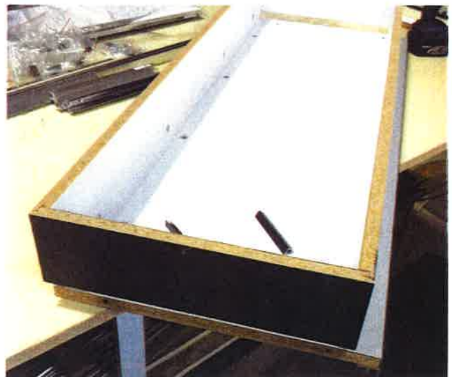
SIDE PANELS ATTACHED TO BOTTOM BASE
