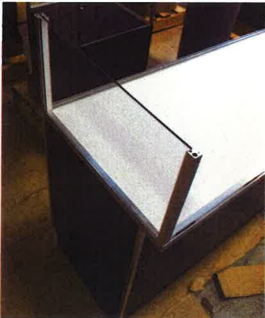
GLASS PANELS INSERTED INTO SIDE FRAMES
