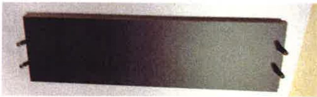
CAM LOCKS INSERTED IN SIDE PANELS
